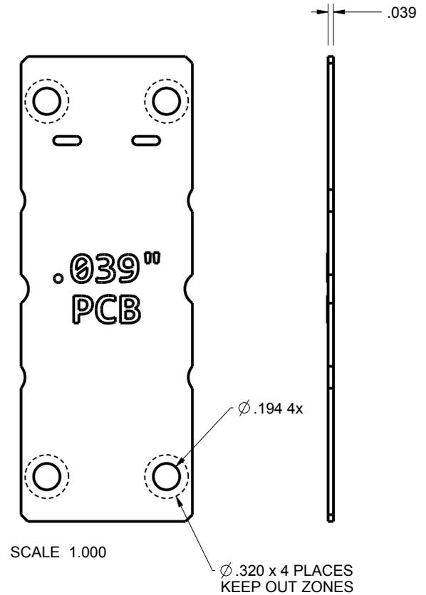
THIS ENCLOSURE CAN ACCOMODATE EITHER PCB THICKNESS
